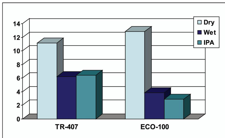
RHOPLEX™ ECO-100 has performances close to a conventional self-crosslinking binder without the associated formaldehyde emissions or residual formaldehyde in the final nonwoven.
