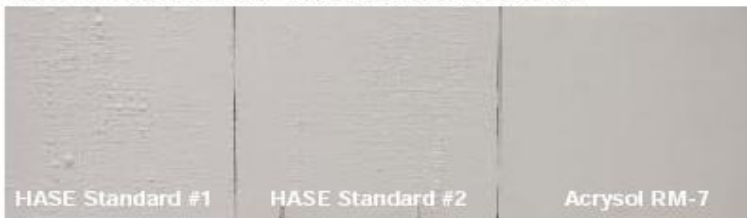
Figure 2 Early Blister Resistance (gloss alkyd, 2 coats/1 day dry/1 hour fog box)
