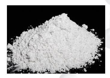
Purmol adsorbents are synthetic zeolites in powder form with a complex alkali aluminosilicate structure. This structure is very open in nature and contains pores of a regular and precisely defined size. This allows for a selective adsorption of molecules based on molecular size and polarity.
