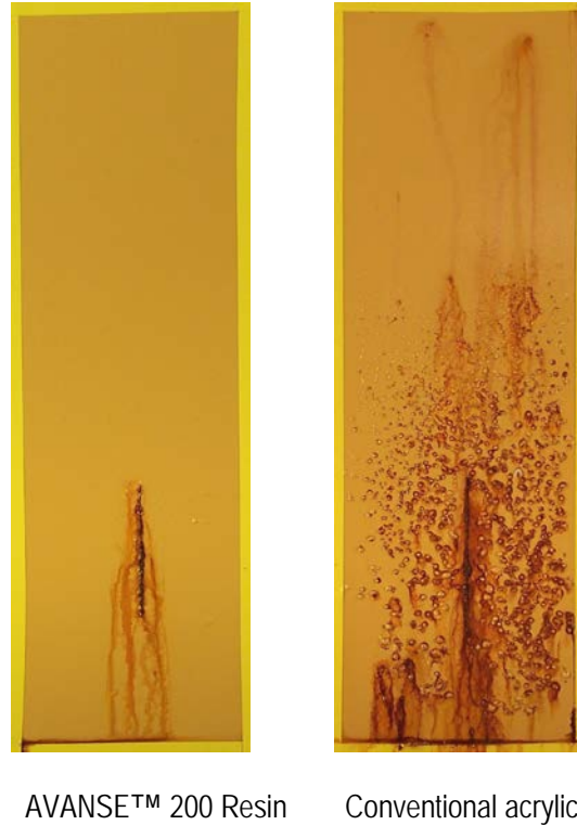
Figure 8. Salt spray resistance at 336 hrs exposure for 9 PVC gloss yellow DTM formulations applied at 3.0 mils DFT on blasted hot rolled steel.
