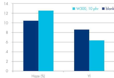
Formulation (phr): PVC Kw62: 100, tin maleate: 2.1, internal lubricant: 0.8, ESBO: 1, Plastistrength® 550 PA: 2, Plastistrength® L1000 PA: 0.15, oxidised PE wax: 0.15, UVA: 0.3
