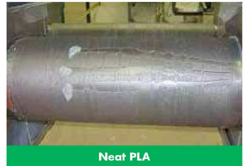
PLA ON A TWO ROLL MILL AT 160°C
