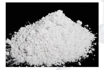
Purmol adsorbents are synthetic zeolites in powder form with a complex alkali aluminosilicate structure. This structure is very open in nature and contains pores of a regular and precisely defined size. This allows for a selective adsorption of molecules based on molecular size and polarity.
